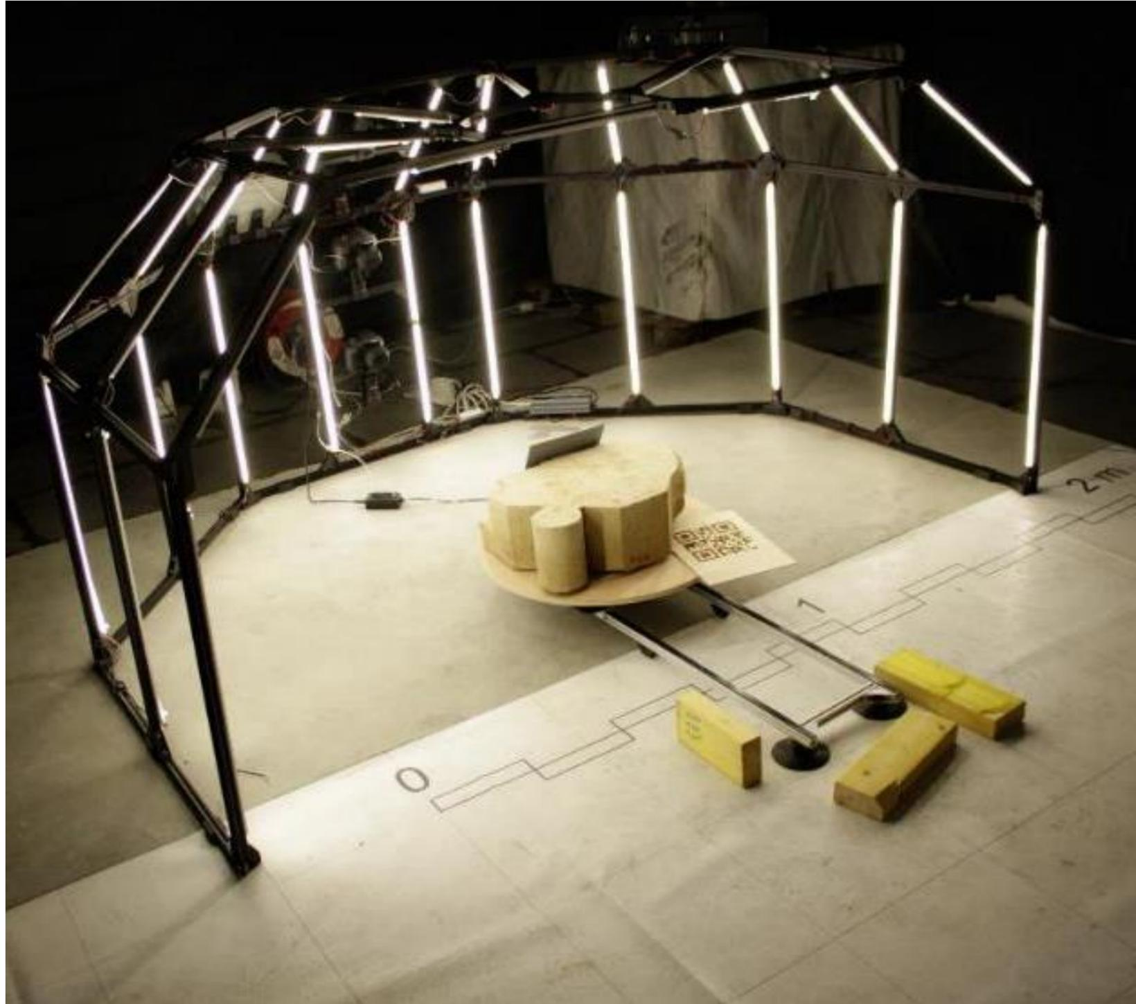
The stones were digitized using a custom photogrammetric rig
