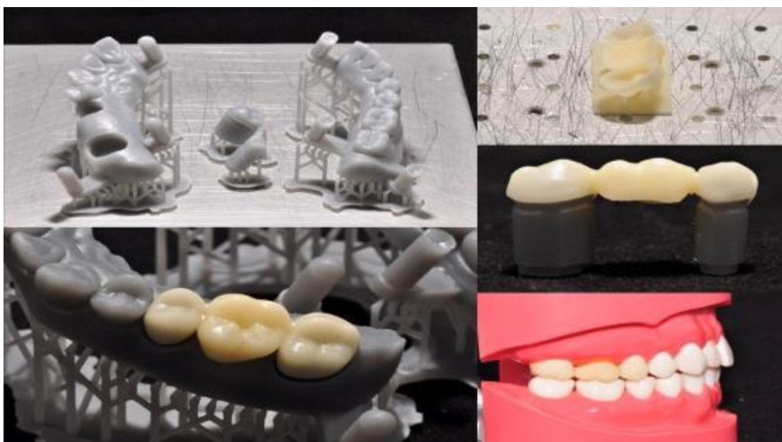
Figure 24 Provisional prosthesis and model can be manufactured on the day of tooth preparation at the dental clinic
